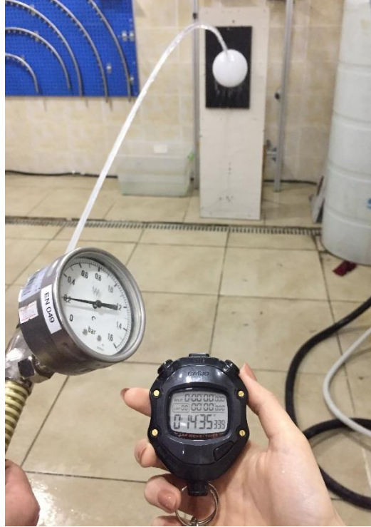
Photo 17. Test condition of model LEDLIGHT-2 for IP X5 test
