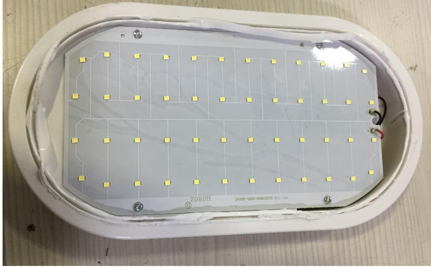
Photo 8. Inside of view after the IP 6X test
