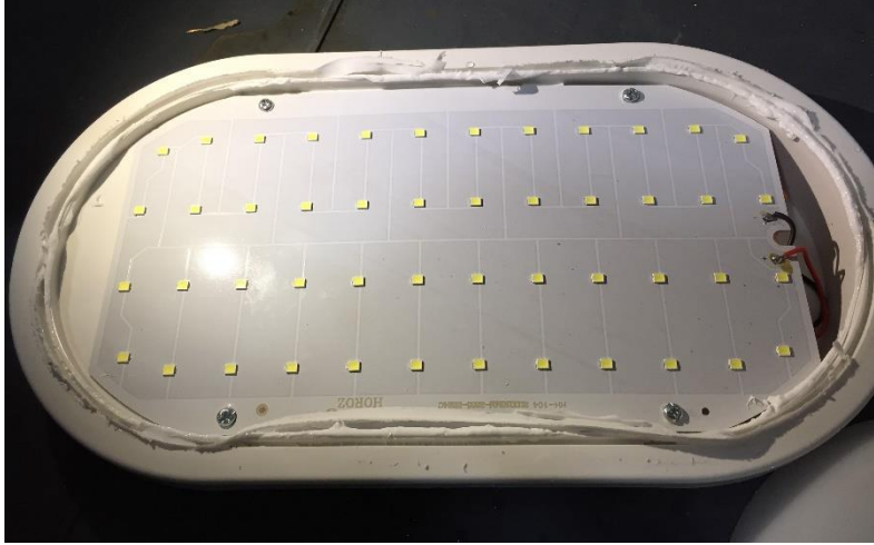
Photo 15. Inside of view after the IP X5 test
