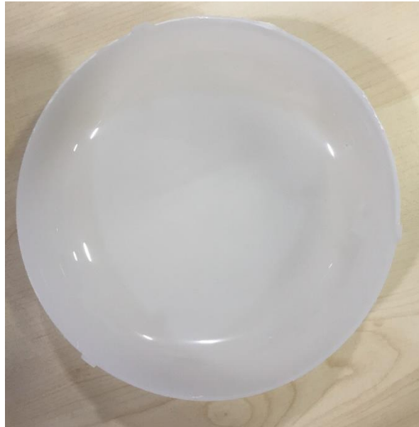
Photo 20. Inside of view after the IP X5 test
