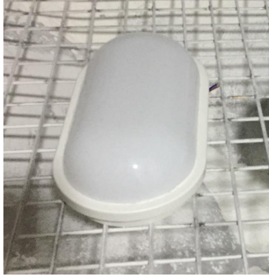
Photo 5. Test condition for IP6X
