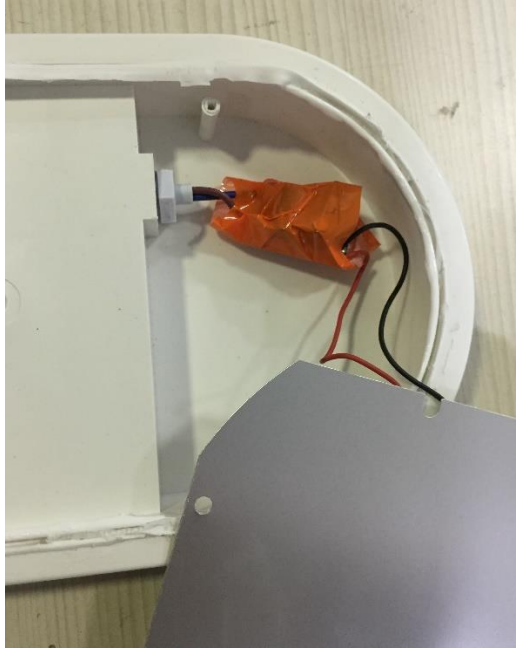
Photo 8. Internal wiring of the product
