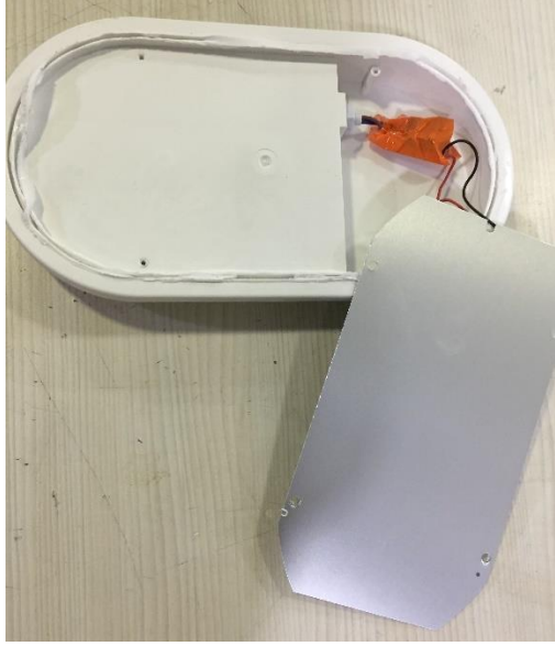
Photo 7. Inside of view after the IP 6X test
