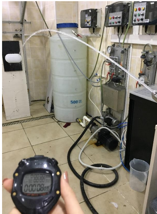
Photo 14. Test condition of model LEDLIGHT-4 for IP X5 test
