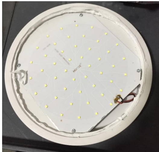
Photo 18. Inside of view after the IP X5 test
