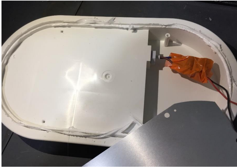
Photo 16. Inside of view after the IP X5 test
